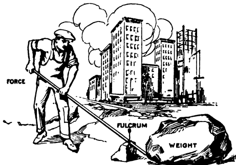
Leverage Needed in Lifting a Stone
